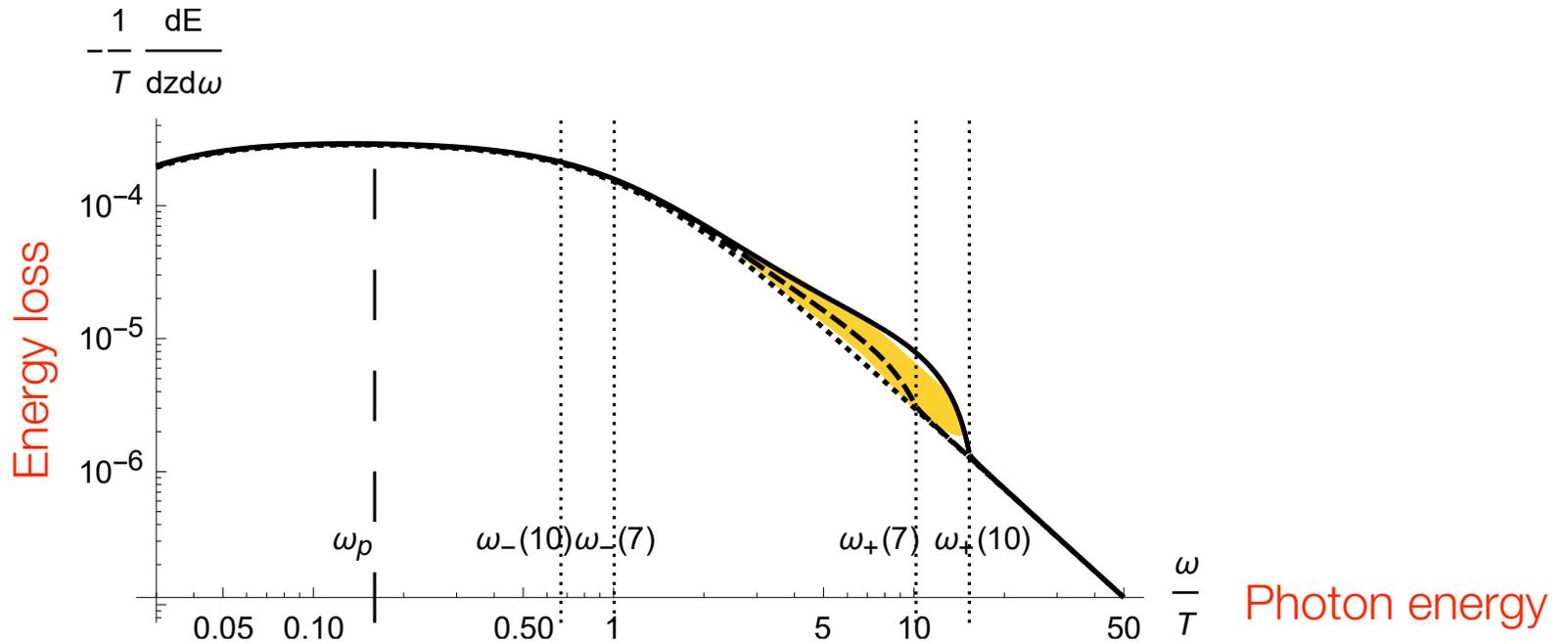
FIG. 1. **Electromagnetic part** of the collisional energy loss spectrum of a  $d$ -quark with  $\gamma = 20$  in Quark-Gluon Plasma. Plasma parameters:  $\omega_p = 0.16T$ ,  $\Gamma = 1.11T$  [36],  $m = T = 250$  MeV. Solid line:  $\sigma_\chi = 10$  MeV, dashed line:  $\sigma_\chi = 7$  MeV, dotted line:  $\sigma_\chi = 0$ .  $\omega_\pm$  are defined in (13).
