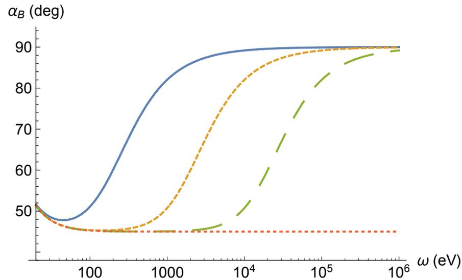
FIG. 2. Brewster's angle as a function of the wave frequency for a typical value of the plasma frequency  $\omega_{pl} = 10$  eV at different values of  $\tilde{\theta} = 10^{-1}, 10^{-2}, 10^{-3}$  (left to right). The dotted line corresponds to  $\theta = 0$ .
