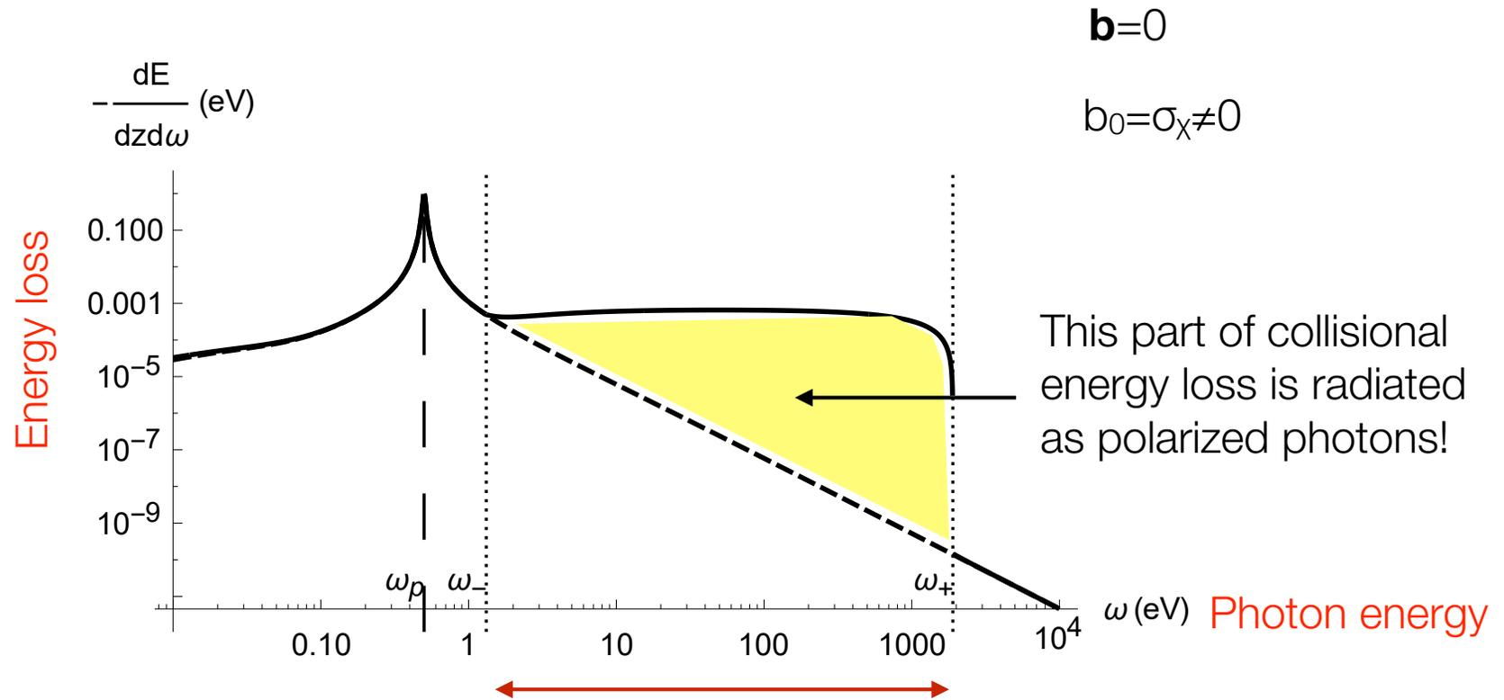
FIG. 2. Collisional energy loss spectrum of electron with  $\gamma = 100$  in a semimetal with parameters  $\omega_p = 0.5$  eV,  $\Gamma = 0.025$  eV (so that its conductivity is 10 eV at room temperature) [41] and  $m = 0.5$  MeV. Solid line:  $\sigma_\chi = 0.19$  eV [42, 43], dashed line:  $\sigma_\chi = 0$ .  $\omega_\pm$  are defined in (13). The seeming discontinuity at  $\omega = \omega_+$  is a visual artifact.
