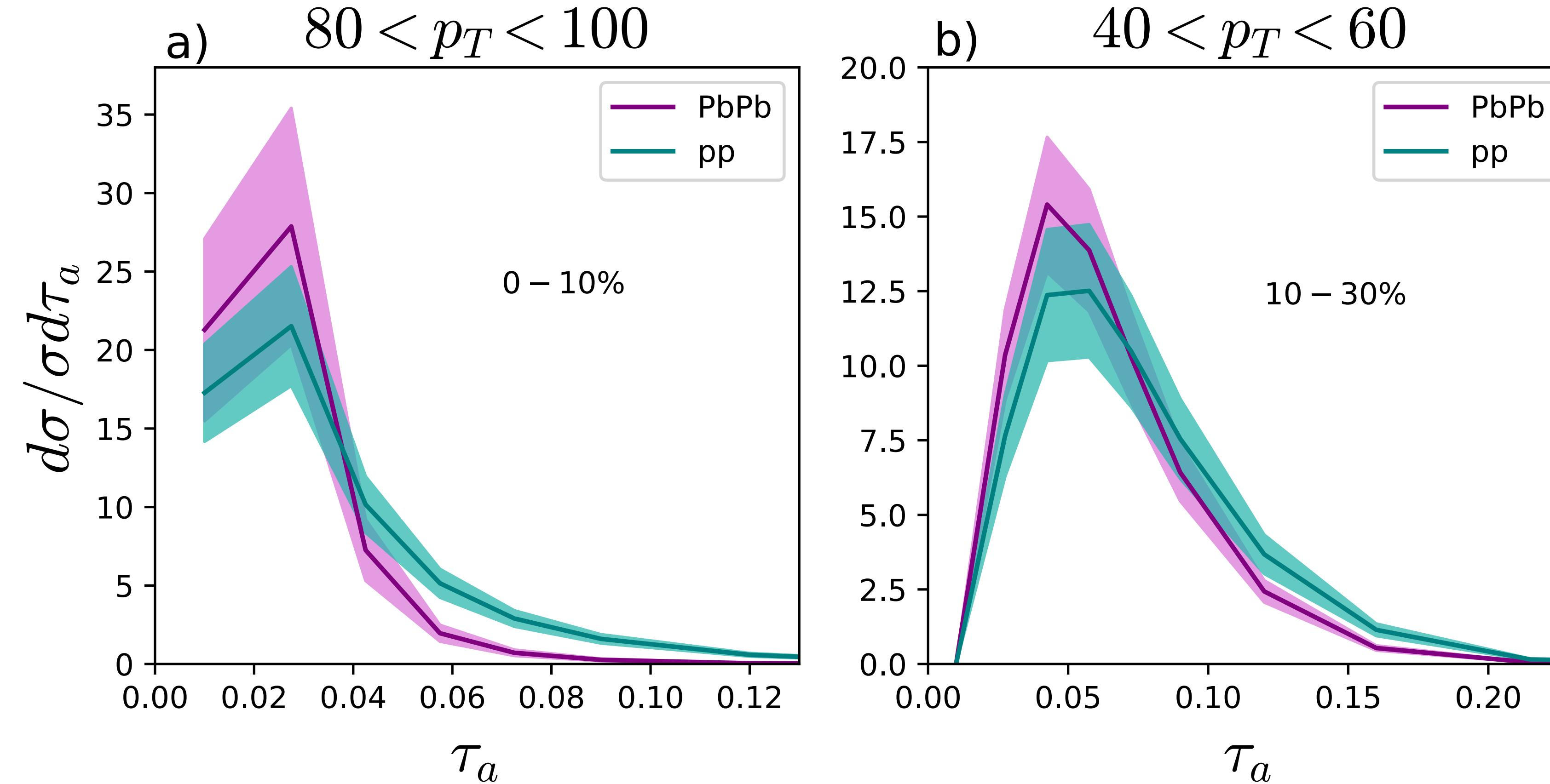
Normalised angularity distributions for  $a = 0$  with (a)  $80 < p_T < 100, 0 - 10\%$  centrality and (b)  $40 < p_T < 60, 10 - 30\%$  centrality, for a jet with  $R = 0.4$
