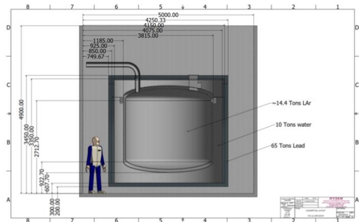
10-ton Argon Cryostat Concept, IU
