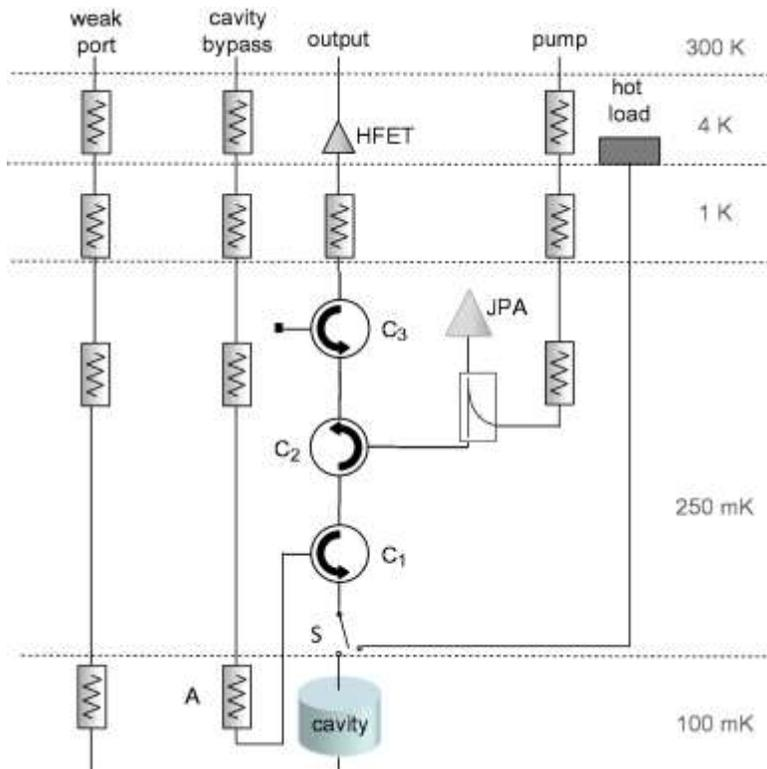
The JPA is tuned to match the cavity frequency
