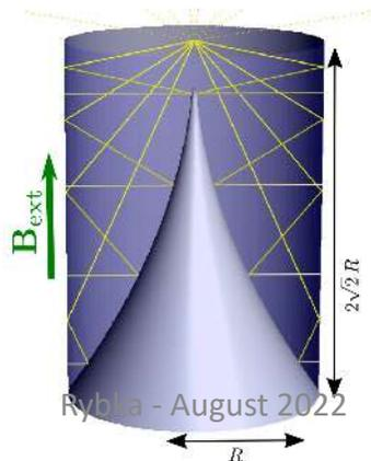
BREAD – folding an axion dish antenna to fit in a solenoid. 240 GHz+. Liu et al. Phys. Rev. Lett. 128 (2022) 131801
