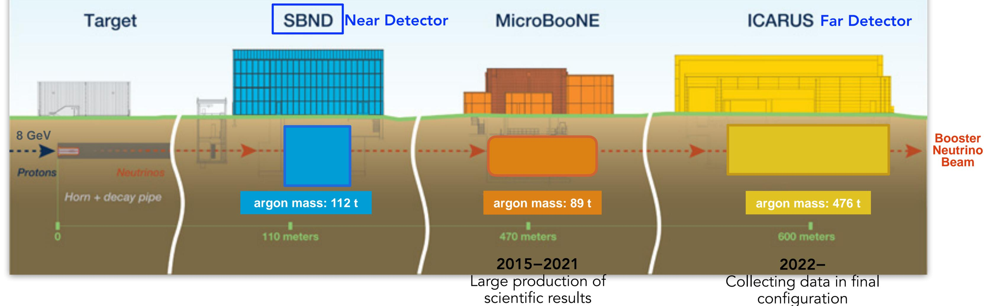
A program designed for **Sterile Neutrino** searches: same **neutrino beam**, **nuclear target** and **detector technology** to reduce systematic uncertainties to the % level.
