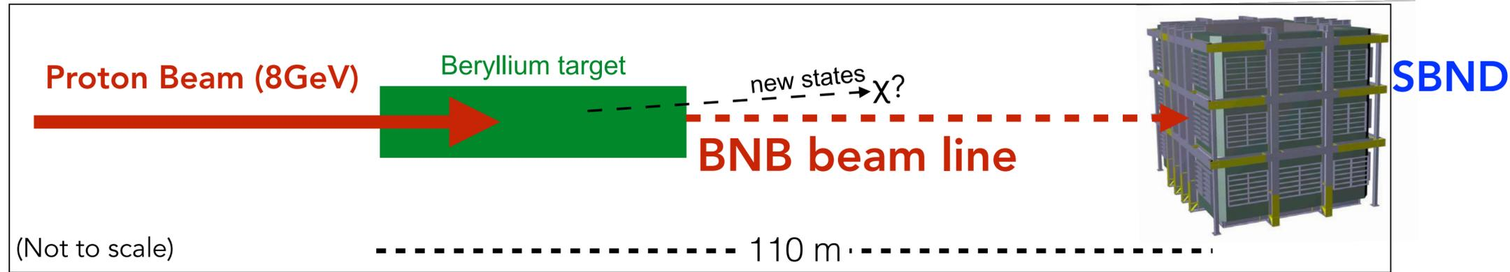
Large mass LAr detector close to the beam target
