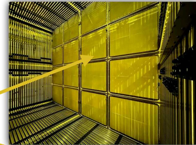
CPA-Cathode covered with TPB coated reflectors
