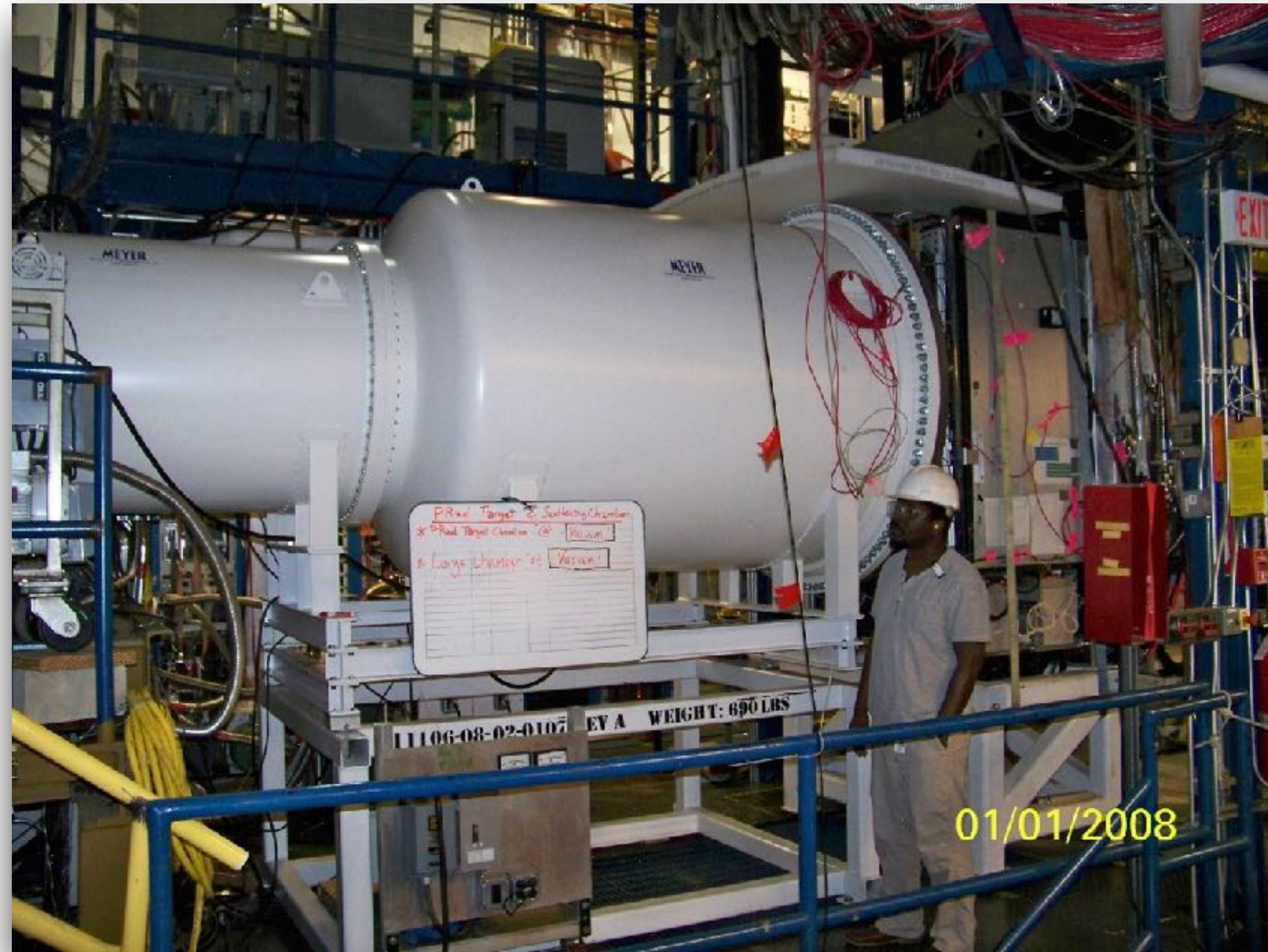
two stage, 5 m long vacuum chamber
