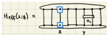
One performs the minimization 1 (or 2) sites at a time, moving across the chain in sequence. The eigenvalue  $\lambda$  converges towards the ground state energy as this is iterated.
