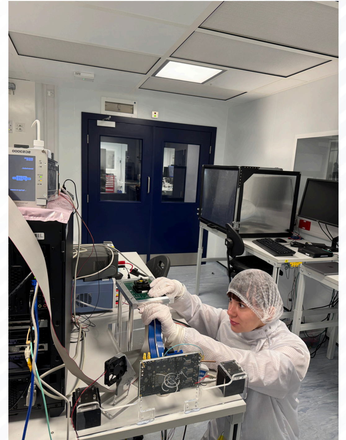
Probe station for sensor testing
