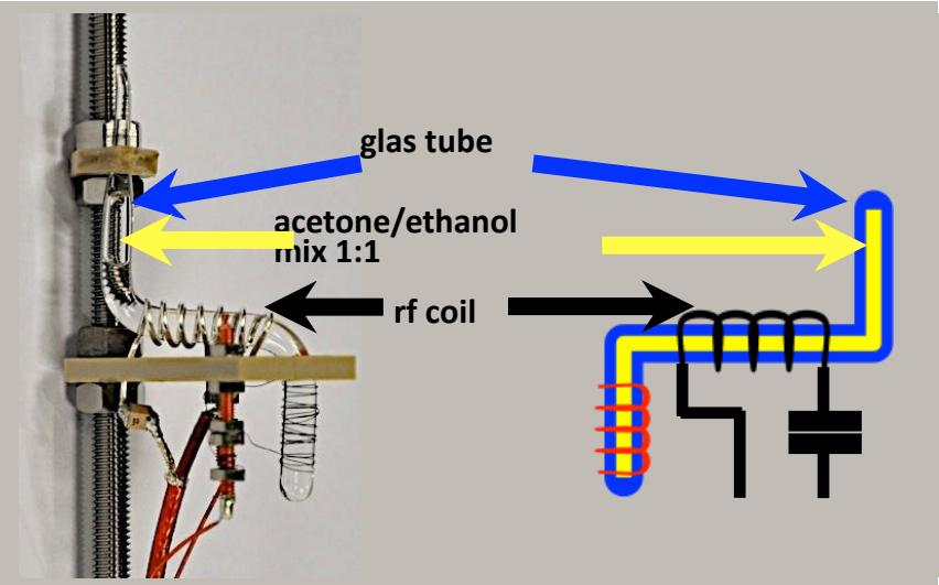
Two probes mounted at electrode system:
