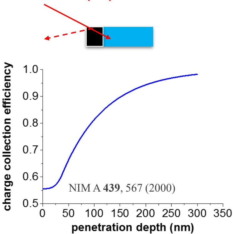
Charge collection efficiency in active layer of similar detector
