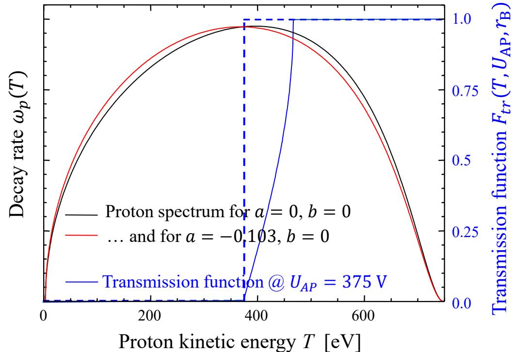
Transmission function  $F_{tr}(T, U_{AP}, r_B = B_A/B_0)$  in the adiabatic limit:
