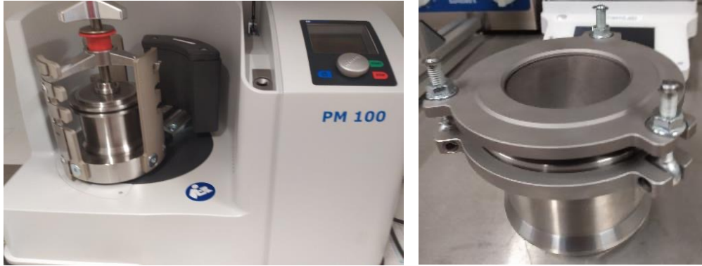
Planetary ball mill – Powder particle size reduction
