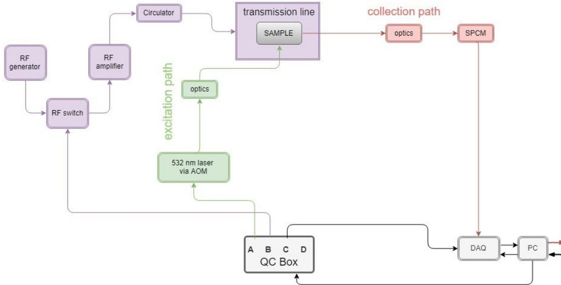
The sample is excited by a 532 nm laser, which drives the nitrogen-vacancy center's spin state to the  $m_s = 0$  ground state and emits a photon ranging between 637- 850 nm. The photoluminescence of the NV center is then redirected through the collection path and the emitted photons are counted. After the spin state is initialized with the laser, the radio frequency (RF) signal is used to drive the spin state to  $m_s = \pm 1$ , which can be observed by a reduction in photon counts.
