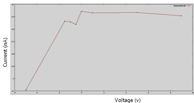
Figure 14: Photocurrent measurement taken from -5V to 5V potential difference from the electron gun using the new DAQ system. Both represent the same data, however the second graph is easier to read with the lines.
