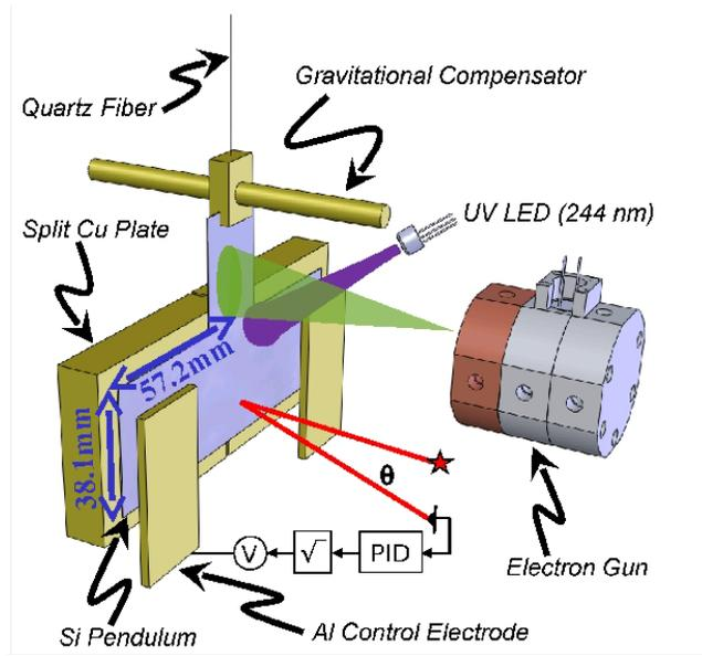
Figure 2: Torsion pendulum that makes up the test masses on either arm of LISA.
