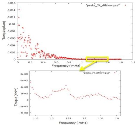
Figure 16: LISA autocollimator data. We observed that the sensitivity is only  $\sim 10^{-8}$  rad/ Hz $^{-1/2}$  where our goal is  $10^{-9}$  rad/ Hz $^{-1/2}$ .
