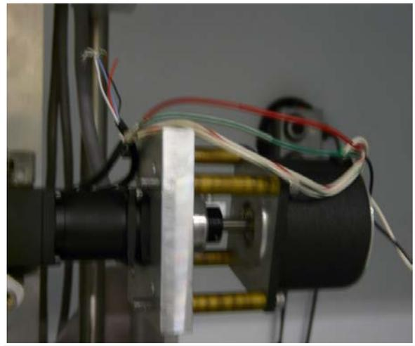
Figure 5: 23D- standard stepper motor replacement. Mounting devices was designed and built at CENPA.
