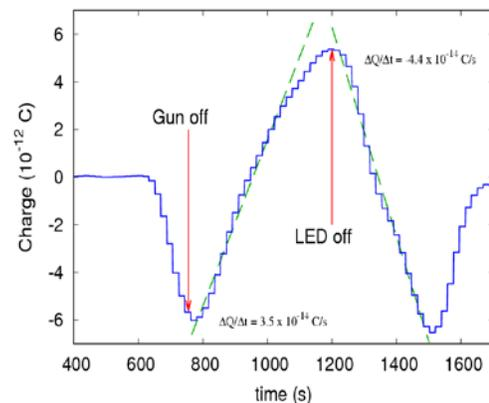
Figure 3: Demonstration of charge control. As the electron gun and UV LED are turned on and off we are able to control the change in charge of the pendulum which is on the order of 0.01 amps.
