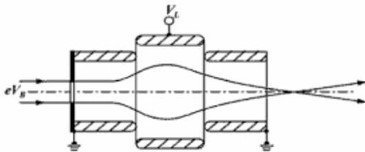
Figure 9: Einzel lens. If  $V_L = V_b$  then the focal length is twice the diameter of the lens. Our design allows the electrons to travel up the gun at the same speed that they were ejected from the magnesium. Figure from *Applied Charged Particle Optics* pg. 42.
