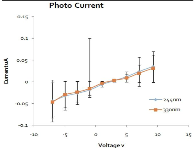
Figure 11: Photocurrent measurement taken with both 240nm and 330 nm UV LEDs on the new electron gun design.
