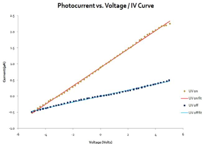
Figure 7: Photocurrent measurement from my electron gun design (see figure 6).
