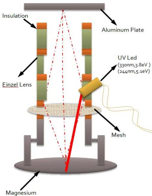
Figure 10: Cross sectional diagram of new electron gun design. Path of photons and electrons are indicated and it can be seen that by incorporating an Einzel lens we can control the flow of electrons to our aluminum measurement plate.
