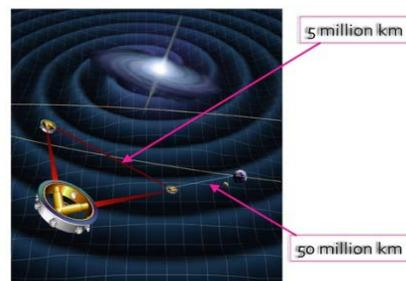
Figure 1: LISA Schematic which shows the layout of LISA relative to the earth and sun. Lasers are reflected off of test masses that are housed in three different spacecrafts.
