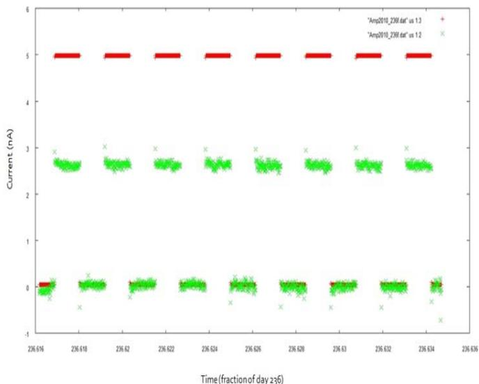
Figure 11: Photocurrent measurement taken with both 240nm and 330 nm UV LEDs on the new electron gun design.
