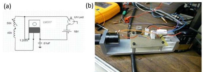
Figure 12: (a) Circuit diagram of battery system. (b) Actual battery system.
