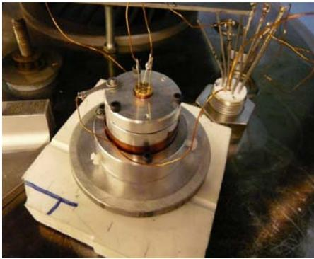
Figure 6: Electron gun to measure photocurrent of our UV LED. The bottom plate is the magnesium cathode while the LED sits on the aluminum cylinder. Different potentials are applied to each component and the photocurrent is measured at the lid.
