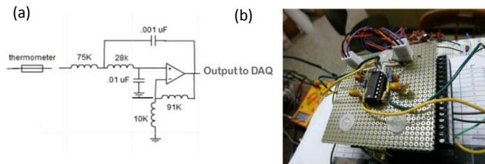
Figure 17: (a) Circuit diagram of thermometer system. (b) Actual thermometer system.
