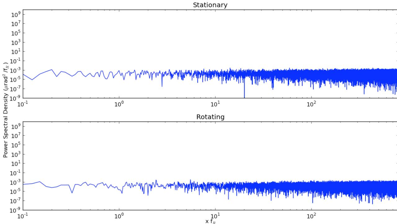
FIG. 6. Two frequency spectra produced by attaching a 9 V battery through the slip ring, a component that allows rotating wires to be connected to a stationary mounting. Data were taken both with the shaft stationary and rotating, revealing that no rotation dependent tilts are present, and that the overall noise level is well below that of the tilt sensor output.
