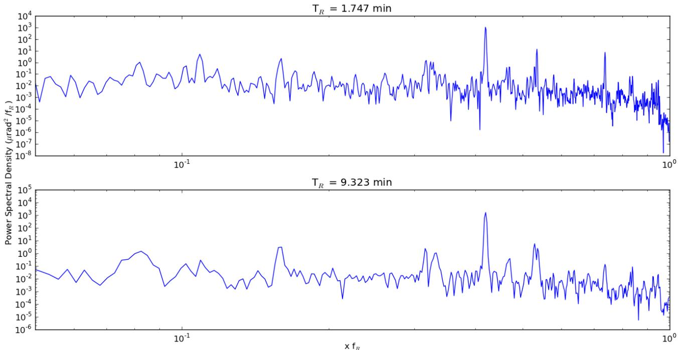
FIG. 5. Two frequency spectra from tilt data measured along one axis with shaft rotation periods of 1.747 minutes and 9.323 minutes. Each spectrum encompasses approximately 16 continuous hours of data, collected over a week apart. Both spectra are in terms of the shaft revolution frequency, revealing several notable ball bearing rotation dependent periodic tilts.
