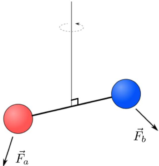
FIG. 1. An illustration of the principle of the torsion pendulum experiment. A pendulum hangs from a thin wire. A twist is induced when a field gradient exists across the pendulum, creating a different horizontal component of force on one side than on the other. The sensitivity of this device allows a well known nonuniform gravitational field to be studied in order to test classical theories of gravity.
