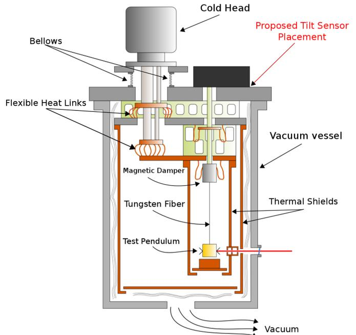
FIG. 2. A schematic of the cryogenic torsion pendulum experiment. The entire experiment is approximately 1 m in height, with a mechanical cold head mounted atop the vacuum chamber that holds the pendulum. The pulse tube cooler cools the pendulum to liquid helium temperatures and remains vibrationally isolated from the rest of the experiment using compressible bellows and flexible thermal links. A tilt sensor apparatus, in development, is proposed to be mounted to the top of the vacuum flange.
