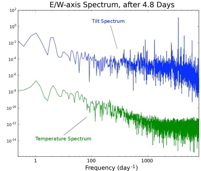
FIG. 8. Spectra created from 4.8 days of tilt and temperature data, revealing the higher frequency rotation dependent periodic tilts, as well as a possible daily and twice daily signal tied to temperature fluctuations.
