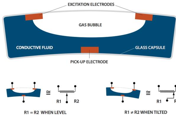
FIG. 3. The principle of operation of the commercial sensor used to measure tilt. A gas bubble is contained along with a conductive fluid. As the sensor is tilted, the bubble moves from side to side changing the resistance between the excitation electrodes and pickup, which changes the voltage output. (Source: *Applied Geomechanics*)
